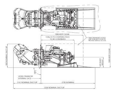
IMPORTANT NOTES: The HTX42 dimensions shown above are <u>Indicative and Preliminary dimensions</u> <u>only</u> for initial design purposes, and subject to change without notice or obligation. Please consult with the factory before using these preliminary dimensions for final installation requirements as these may have changed.
